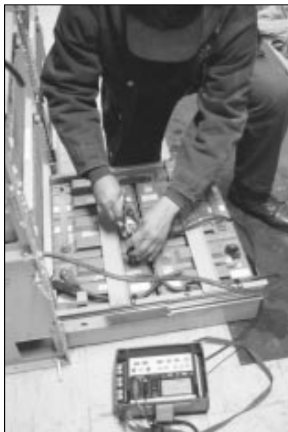
Taking direct intercell connection resistance measurements with the C-BITE.
