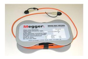
The patchcord connector must be representative of the type and quality of those used to connect the link during its normal operation. This is the only way to accurately assess the quality of the near end link connector.
